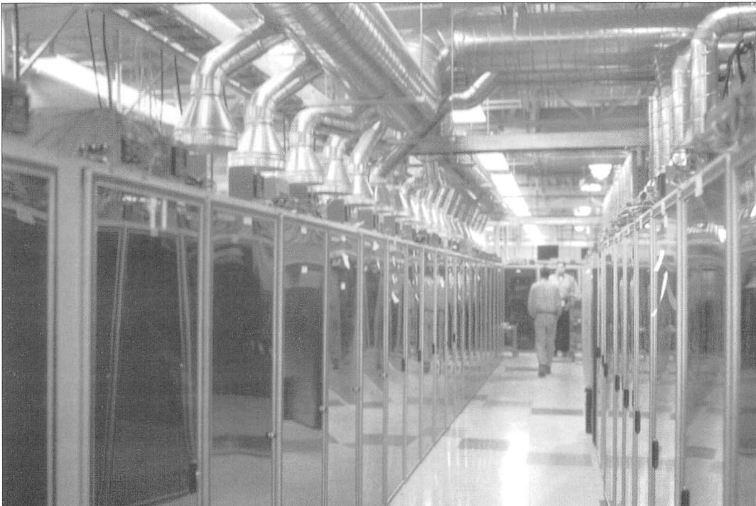
Products are quality tested by placing them in thermal burn-in centers.
