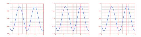
Now think of these as "frames" in a TV/Video signal. These frames are successively superimposed over each other. As their starting point is the same and the signal is a repetitive signal, we get the same pattern in each sweep. Therefore we can see a steady image on the screen.
