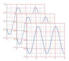
You can imagine that playing these frames successively will result in a steady image as opposed to one that is moving across the screen. Now you can make measurements of frequency and amplitude.
