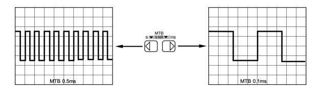
Pressing the MTB button. We will see that the scale for the graticles is shown below on the screen and changes as we press this.
