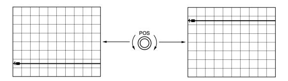
2. Now move to DC coupled mode. Measure the position compared to the GND coupled position in terms of the graticle. Let's say we get graticle 5/8. That means we have a voltage of 3V as we are 3 graticles away from the GND and each graticle is 1V apart.
