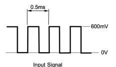
With this signal, the oscilloscope can calibrate all channels automatically. Before the start of your experiment you should do this.
