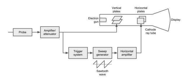
**Probe:** The piece that connects to your circuit under test. Most probes have two tips, as oscilloscopes measure the electric potential difference (voltage) between two points.
